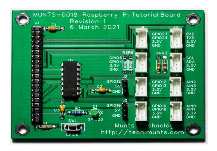
It contains an on-board A/D converter, an LED, a momentary switch, two 3-pin 5V servo headers, and 8 <u>Grove System</u> connectors:
